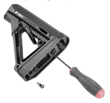
6. Attach an SL pattern recoil pad to the rear of the SAA Lite using the included  $10-24 \times 3/8$ " button head screws. Torque to 15 inch lbs. If using a Limbsaver SL, be aware that the screws must be pushed into the soft pad until the threads protrude from the other side.
