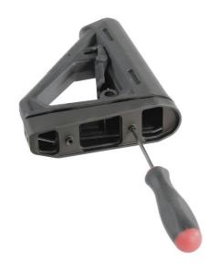
5. Attach the original recoil pad, SL Enhanced pad, or SL Limbsaver to the rear of the SAA Lite using a 1/8" Allen wrench and the included  $10-24 \times 3/8$ " button head screws. Do not exceed 15 inch lbs of torque. If using a Limbsaver SL, be aware that the screws must be pushed into the soft pad until the screw head disappears and the screw threads protrude from the other side.
