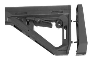
4. Using the same 1/8" Allen wrench, insert it into the threaded holes on the back of the SAA Lite and tighten, making sure to alternate between the top and bottom screws so it evenly reduces the gap between the SAA Lite and stock until snug. If you attempt to tighten the top or bottom completely instead of alternating, it will cause the screws to bind. Do not exceed 15 inch lbs.
