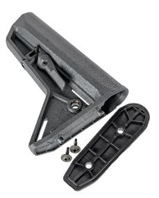
2. Reuse the screws from step 1 to attach the front half of the Stock Angle Adapter to the SL or SL-S stock. Torque to 15 inch lbs.
