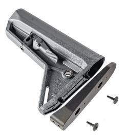
3. Attach the rear half of the Stock Angle Adapter using the provided button head screws. Torque to 30 inch lbs.
