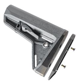
4. Attach the recoil pad to the rear of the Stock Angle Adapter using the provided button head screws. Torque to 15 inch lbs.
