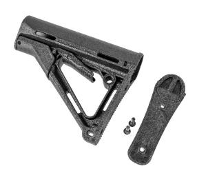
2. Reuse the screws from step 1 to attach the front half of the Stock Angle Adapter to the CTR stock. Torque to 15 inch lbs.
