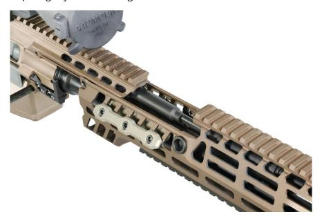
7. Continue to slide the handguard onto the upper receiver. When the handguard is approximately 1/2" from being fully seated, it will be necessary to gently maneuver the clamp on each side inward and upward so that they clear the barrel extension. You will then be able to seat the handguard fully to the rear.
