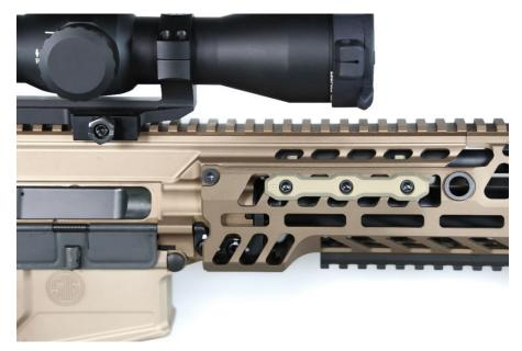
9. Press the ZRC clamps on each side inward toward the barrel and upwards until you see the two hooks on the inner clamps through the upper vent holes, as shown. Continue to hold the clamp in place while tightening the three screws on each side until finger tight.
