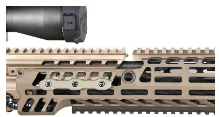
8. Press the front takedown pin into place and install the two new 8-32x3/8" Torx flat head screws into the holes at the rear of the handguard. Torque to 20 inch lbs.
